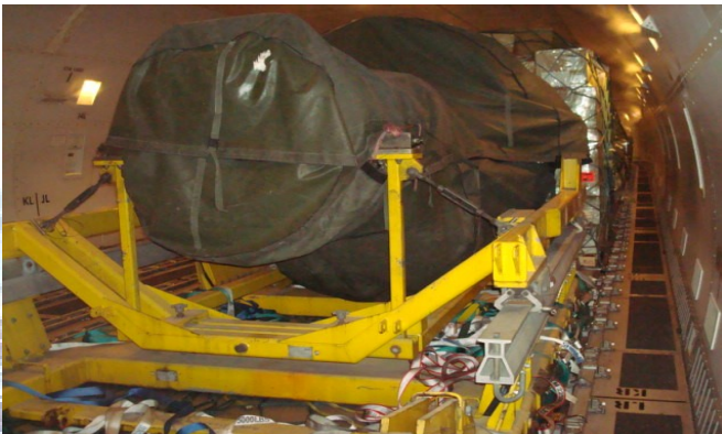
Photos show the loading of a V2530-A5 engine used on the Airbus A320 being transported to New Zealand on 7 Feb 2009
